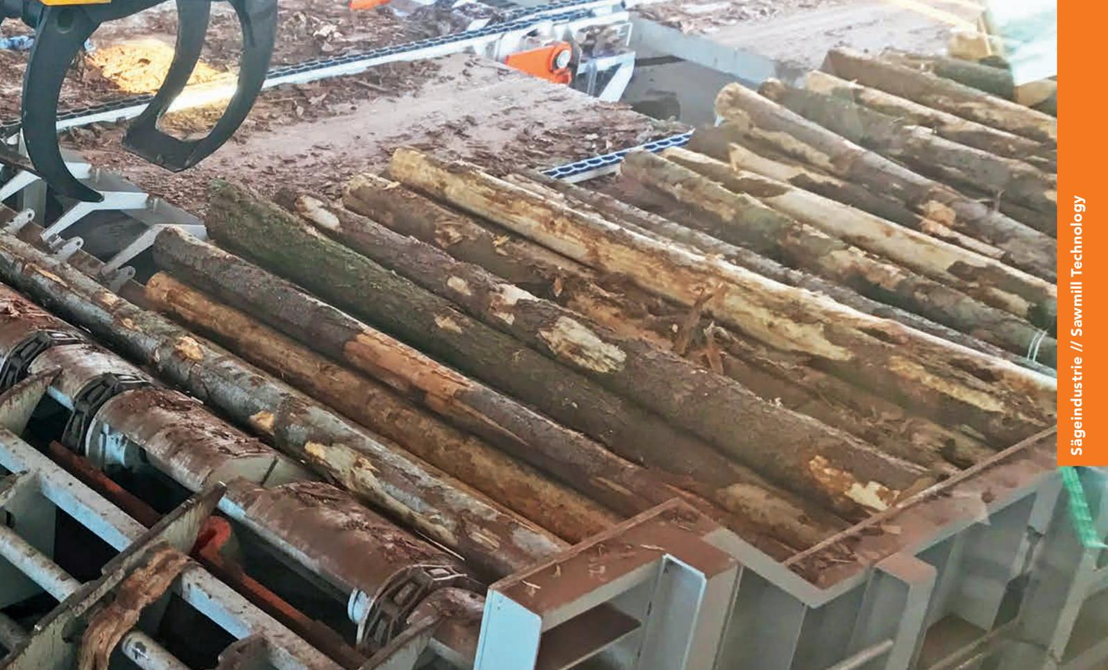
Long and short logs are transferred in parallel to the V-rollerway via electrically controlled feeding units. The well tested Holtec chainless system is used here which works without the high-wear chains. The V-rollerway accelerates the logs and controls at the same time the distance between the logs via the innovative driving concept Gap-Control. Subsequently the logs can be fed to the Valon Kone debarker with a clearly defined gap.
